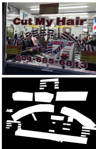
Figure 1: Annotation details of Total-Text, including transcription, polygon-shaped and rectangular bounding box vertices, orientations, care and do not care regions, and binary mask.
