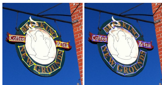
Fig. 8 a Original ground truth with uncontrolled length of polygon vertices. b Our new regulated ground truth with a fixed length of 10 vertices
