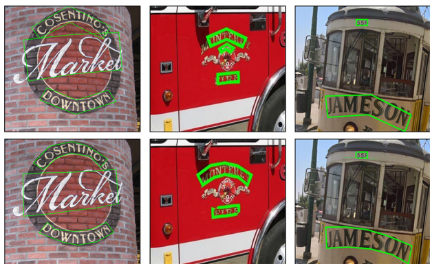
Fig. 21 1st row: Poly-FRCNN-3; 2nd row: Poly-FRCNN-5. Poly-FRCNN-5's output has more vertices, hence, is able to bind curved text with larger curvature more tightly
