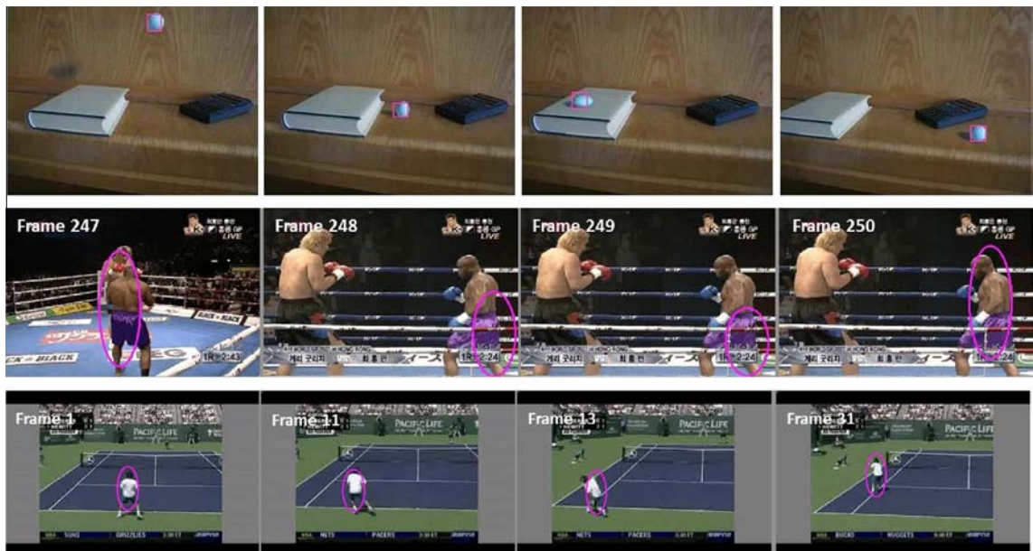
Fig. 1. Example of the abrupt motion in different scenarios. Top: Inconsistent speed. Middle: Camera switching. Bottom: Low frame-rate videos.
