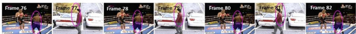
(c) Sample detections by the SwATrack tracking. In Frame 77, since the object-of-interest does not appear in the frame, inaccurate tracking happens. However, the SwATrack is able to recover its tracking at the following frame, Frame 78.
