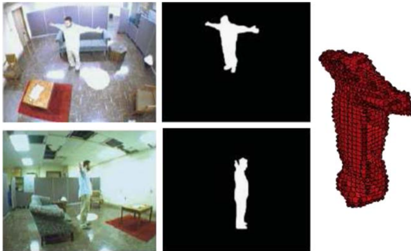
Fig. 11. Voxel person constructed using multiple cameras from different viewpoints of the silhouette images that resolved the occlusion problem in the single camera system. However, due to the location of the cameras and the person's positions, the information gathered using the crisp voxel person model can be imprecise and inaccurate. Therefore, the fuzzy voxel person representation was proposed [104].
