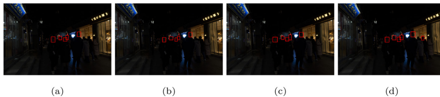
Fig. 13. YOLOv4 detection results on DarkFace-val set with different settings: (a) YOLOv4 trained with DarkFace training set only; (b) YOLOv4 trained with DarkFace training set and (LTFT + FEEDS)-day-to-night-transformed images generated by NICE-GAN; (c) YOLOv4 trained with DarkFace training set and (LTFT + FEEDS)-day-to-night-transformed images generated by MUNIT; (d) YOLOv4 trained with DarkFace training set and (LTFT + FEEDS)-day-to-night-transformed images generated by AugGAN-Det.
