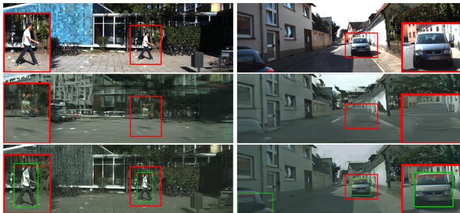
Fig. 14. KITTI-to-Cityscape results: (1st row) original images; (2nd row) detection results in MUNIT-transformed images (pedestrian and cars cannot be detected because they are not preserved during image-translation); (3rd row) detection results (green bounding boxes) of images transformed by this work. (For interpretation of the references to color in this figure legend, the reader is referred to the web version of this article.)
