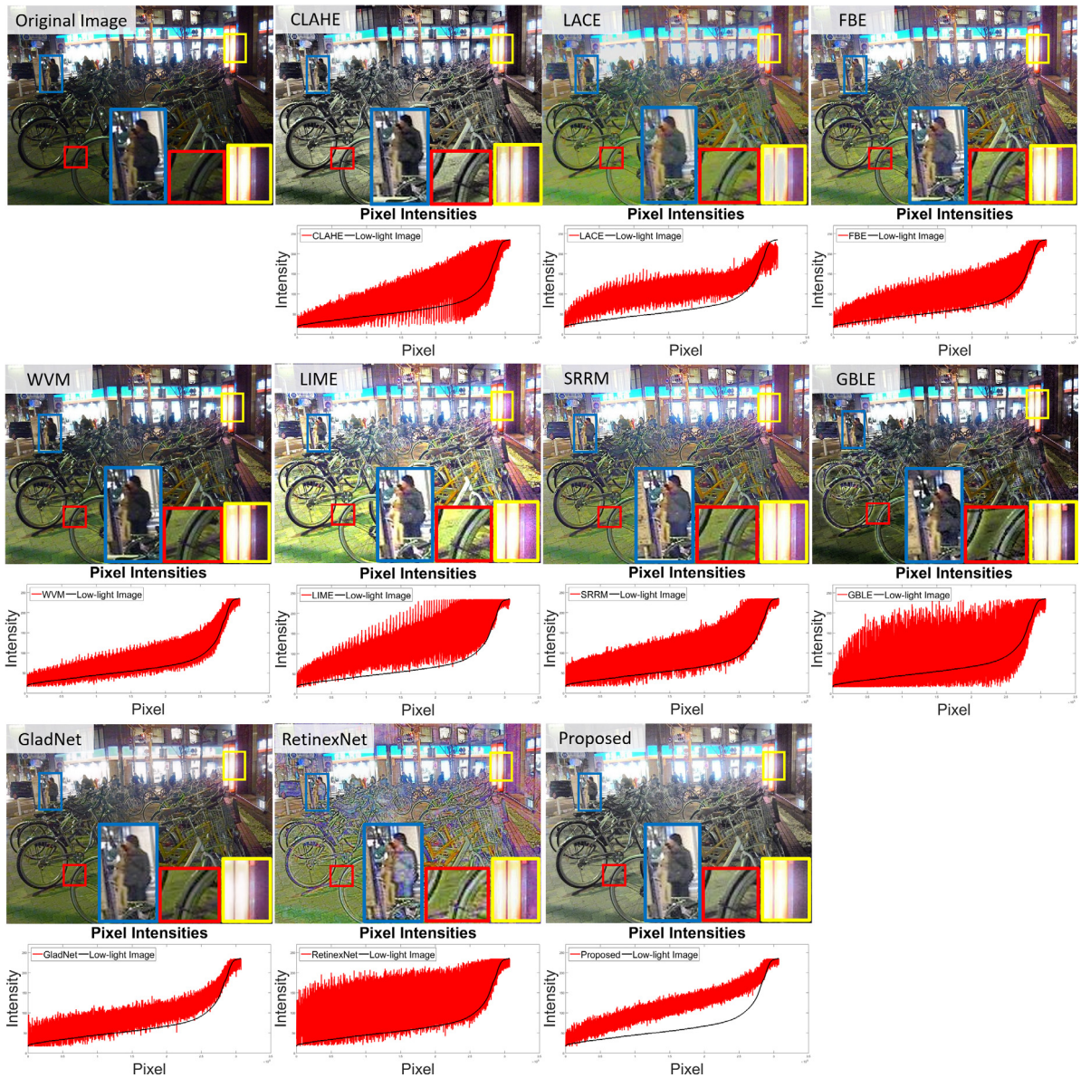
Fig. 10. Example of the contrast enhancement on a real low-light image, and the intensity of each pixel before and after enhancement of the respective methods (arranged in ascending order of pixel values from the original low-light image). [Best viewed in color].
