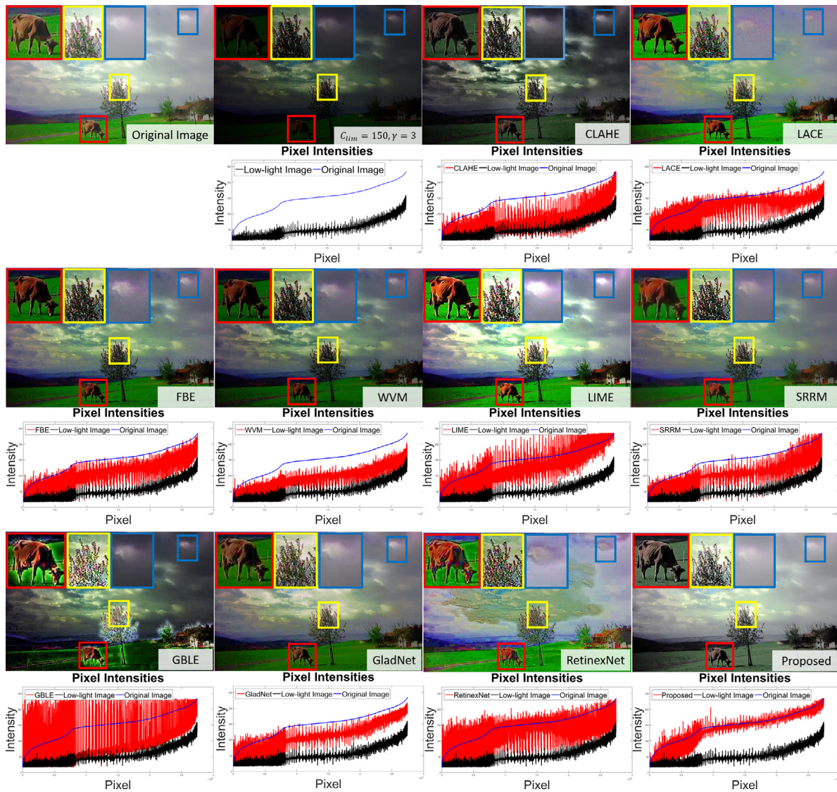
Fig. 11. Example of the contrast enhancement on a synthesized low-light image, and the intensity of each pixel before and after synthesis and enhancement (arranged in ascending order of pixel values from the original bright image). [Best viewed in color].
