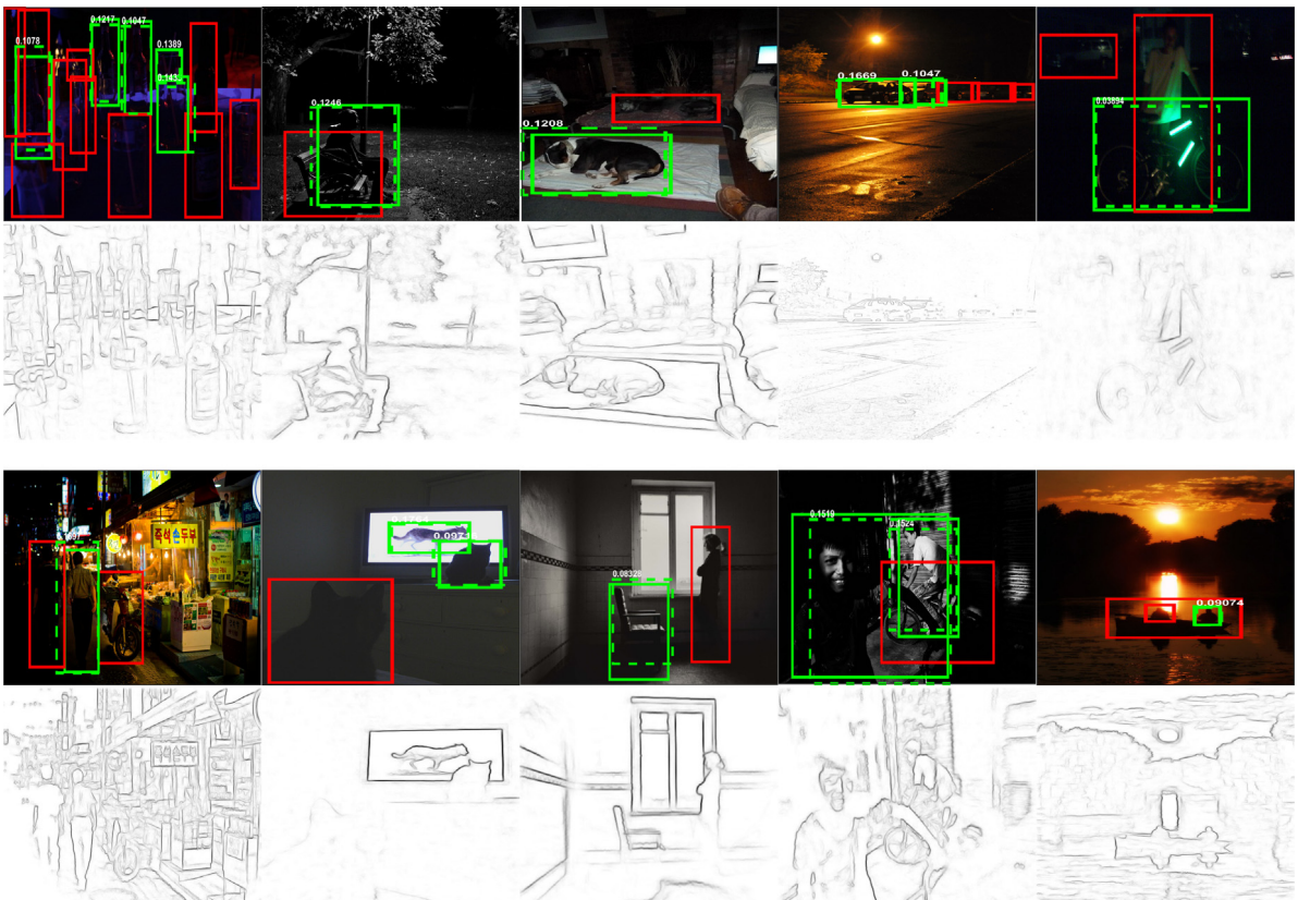
Fig. 8. Examples of Edge Boxes proposals (Max. proposals = 1000; IoU = 0.7) on different types of low-light images (top) and visualizations of their respective edge features (bottom). (Red: undetected groundtruth; and Green: detected groundtruth, Green dotted: proposed box) From left, first row: Low , Ambient , Object , Single , Weak ; and second row: Strong , Screen , Window , Shadow , Twilight . (For interpretation of the references to color in this figure legend, the reader is referred to the web version of this article.)
