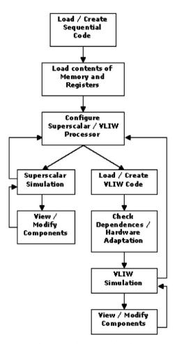
Fig. 1. Typical execution flow.
