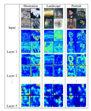
Fig. 3: Visualization of neurons' response in the *genre* classification task. Input neurons represent raw pixel values which are combined to edges in the lower layers (Layer 1). In the middle layers contours of parts thereof are built, which are finally combined to abstract features such as faces (Layer 5).
